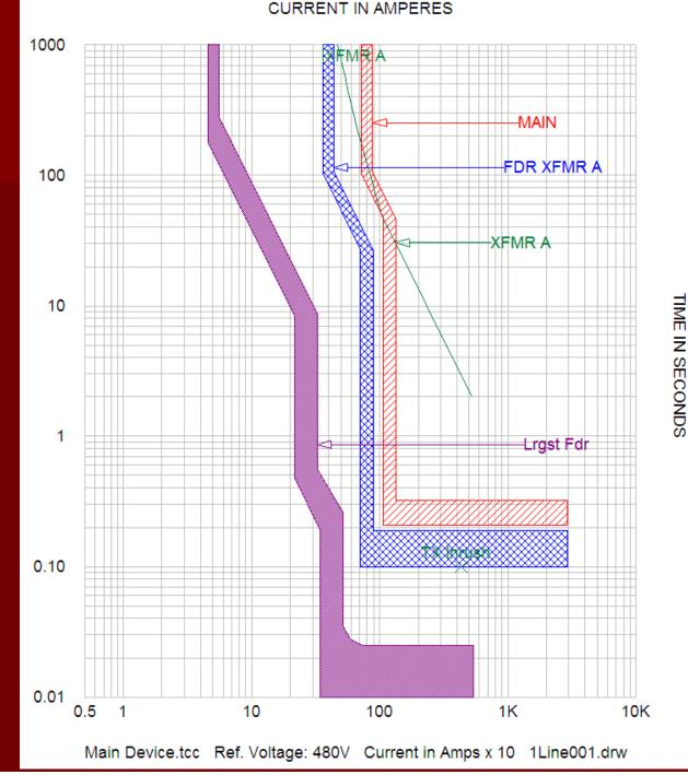
Using Solid State Trip Breakers @ 30 kA Available HRC (Cal/cm<sup>2</sup>)
