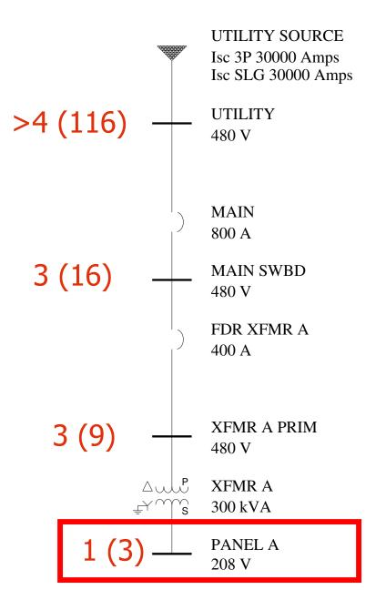
Arcing Fault Current @ Panel A – 5.0 kA Panel A is protected by 400A Feeder Breaker in Main Switchboard Current is reduced due to transformer: - 5.0 kA @ 208 Volts - @ 480 V = 5.0\*208/480 = 2.2 kA Feeder breaker sees only 2.2 kA for a fault at Panel A!!!
