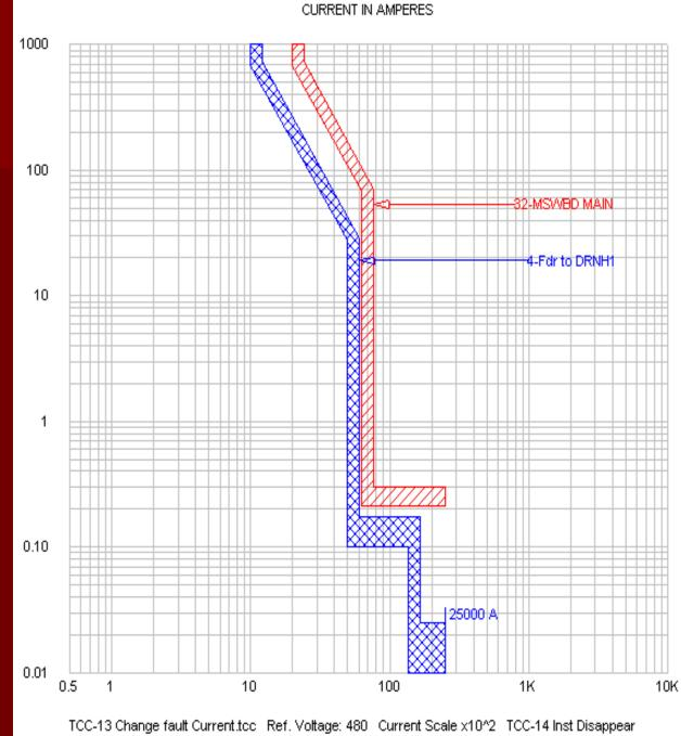
Instantaneous curve ends at available fault current
