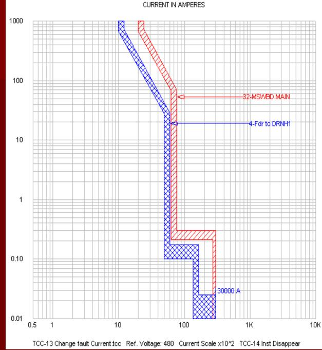
Instantaneous curve ends at available fault current
