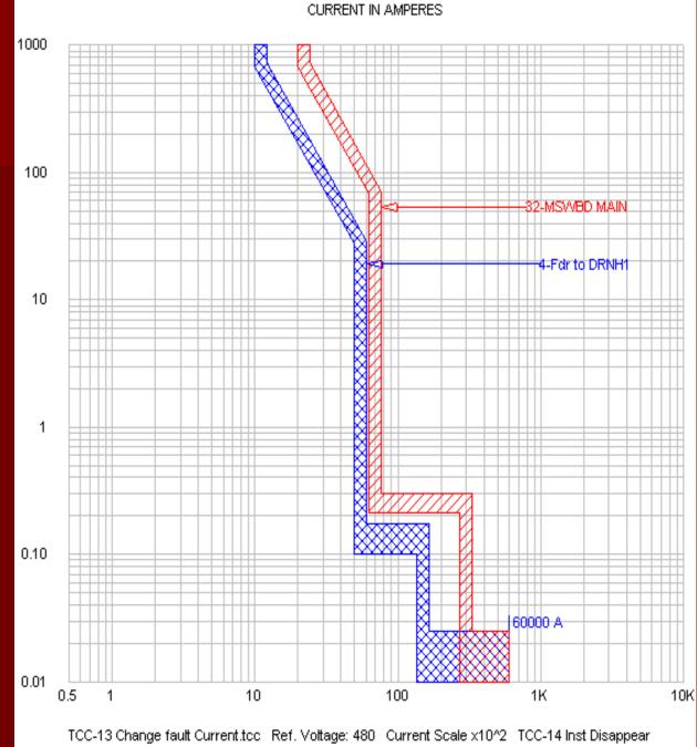
Instantaneous curve ends at available fault current
