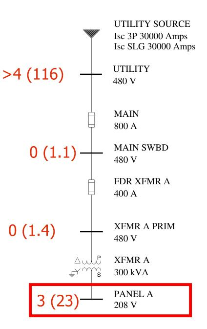
Arcing Fault Current @ Panel A – 5.0 kA Panel A is protected by 400A Feeder Fuse in Main Switchboard Current is reduced due to transformer: - 5.0 kA @ 208 Volts - @ 480 V = 5.0\*208/480 = 2.2 kA Feeder fuse sees only 2.2 kA for a fault at Panel A!!!
