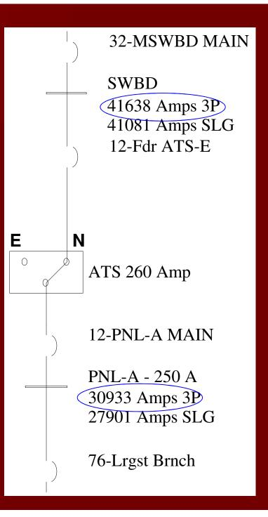
32-MSWBD MAIN SQUARE D NW40H Sensor/Trip 4000 A Settings Phase LTPU/LTD (A 0.4-1.0 x S) 1 (4000A); 0.5 STPU (1.5-10 x LTPU) 5 (20000A) STD (INST-0.4) 0.3(I^2 T Out) INST (2-15 x S) 15 (60000A)
