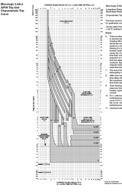
M-frame, P-frame, R-frame and NS630b–NS3200 Electronic Trip Circuit Breakers
