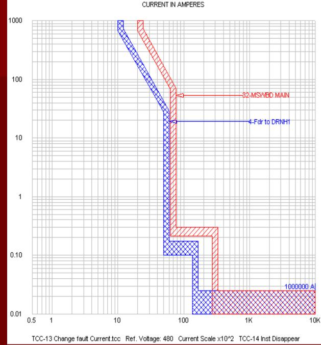
Instantaneous curve ends at available fault current
