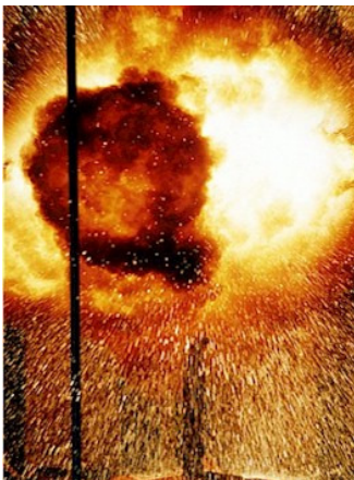
Figure 1 - Arc Flash Accident
